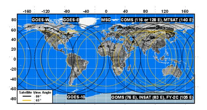
Figure 1. Components of a global geostationary fire monitoring system.
